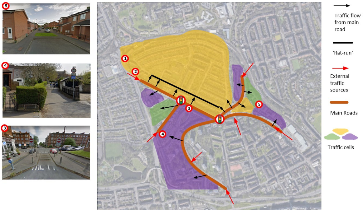
Image showing routes traffic can take around Broomhill. Highlighted are the cells that have been created using modal filters and inset images show these.
