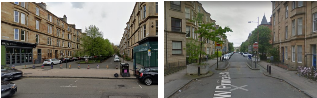
(Left) Continuous walkway created by blocking connection to Great Western Road. This also creates a better walking experience as there is no longer a street to cross. (Right) Modal filter on West Princes Street which stops through traffic using residential streets.
